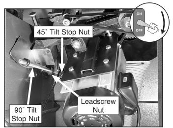
Figure 83. Blade tilt stop nuts.
